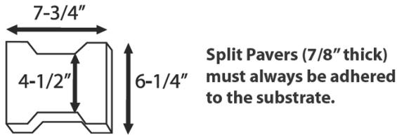
Full Pavers (1-3/4" thick) may be adhered or loose-laid. If loose-laid, pavers must be installed against a perimeter border system (see instructions for loose-laid installation).
