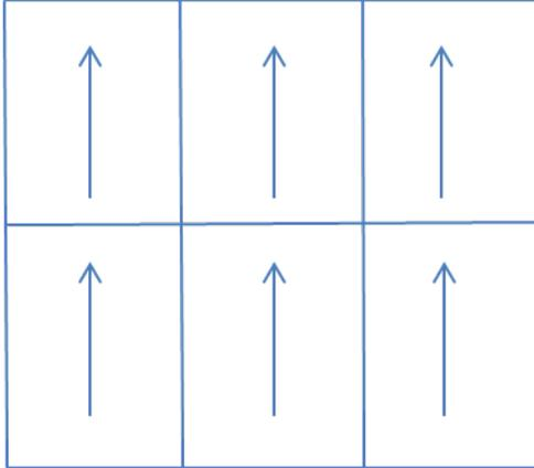
7. PLEASE NOTE: ALL NON-WOOD PATTERNS Strait Rx, Cosmos Rx, and Infinity Rx rolls must be unrolled and installed in the same direction within each consecutive run. Adjacent rows must be laid in the opposite direction to avoid shade variations between the rolls.
