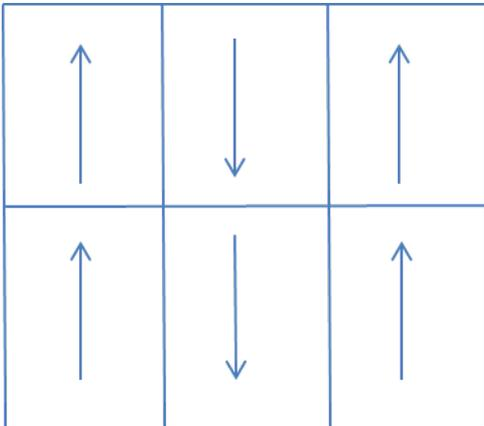
8. Lay the rolls to provide as few seams as possible with economical use of materials. Match edges for color shading and pattern at seams. Be prepared to straight edge cut the side seams to ensure pattern consistency.
